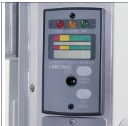
Guardian™ Digital Airflow Monitor
