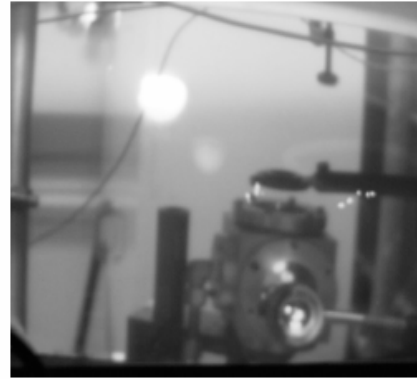
Figure 3.1. IR image of the transmitted laser pulse image on the back wall.
