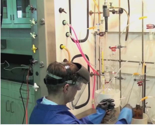
clutter removed nitrile gloves full eye protection face shield (Added) flame-retardant lab coat bottle and reaction vessel clamped containment vent line bubbler 3-5psi inert gas on bottle
